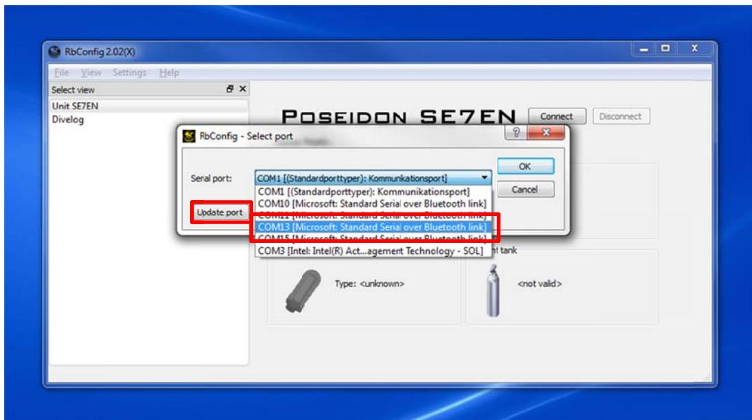
10. The software is now ready to connect to the Poseidon SE7EN. This is easy, just press the connect button.
