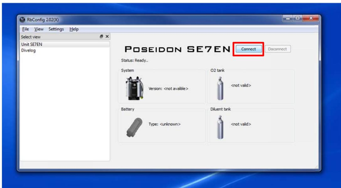
11. The computer now connects to your Poseidon SE7EN (if it is turned on; either by wet switch or by installing the battery) and you can now follow the pre dive sequence in system window, determine your battery type and see cylinder pressures.
